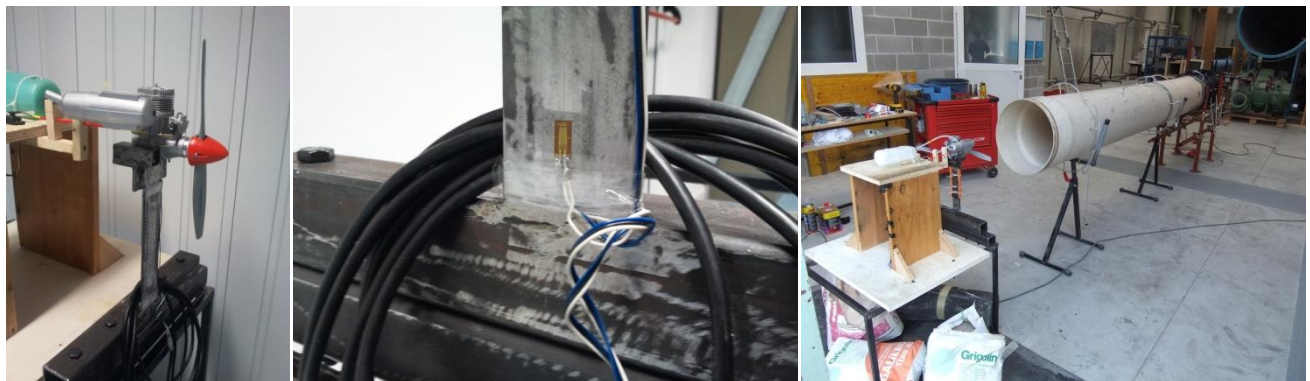
Figure 4: Test rig for propeller thrust measurements, left –engine mounted on the cantilever beam, center- strain gauge, right – the engine placed in front of the open end wind tunnel.
