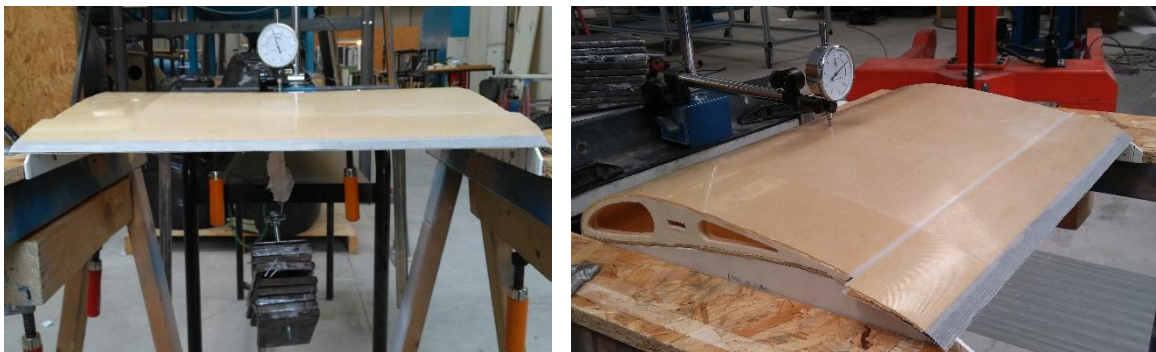
Figure 8. Static load test for the determination of critical deformation (radius of curvatre).
