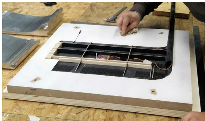
Figure 16. Vertical stabilizer internal structure
