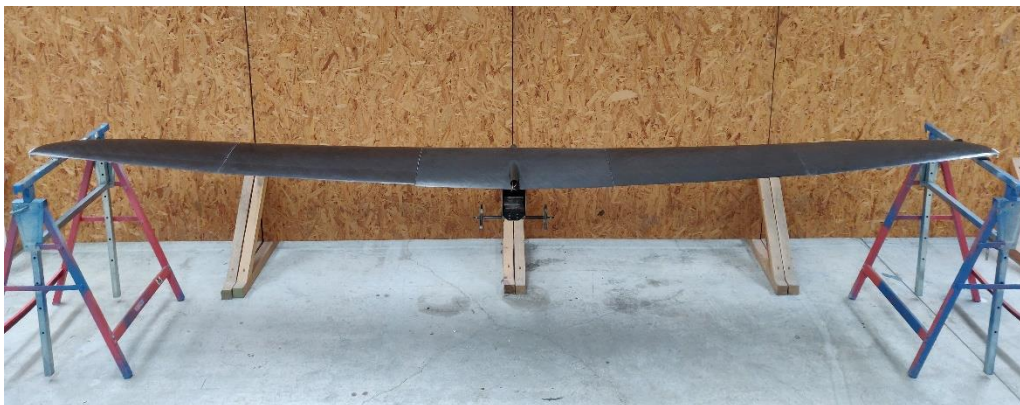
Figure 20: Loading the wing to determine the overall stiffness of the structure.
