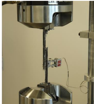
Figure 12: Carbon fibre specimen subjected to a tensile test.
