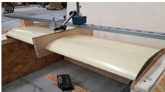
Figure 14: Test bench for deflection (left) and torsion (right) measurements of the wing structure.
