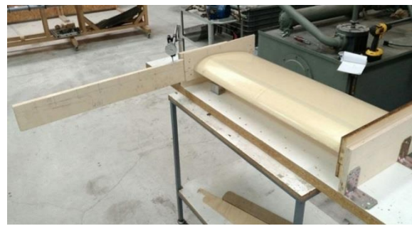
Figure 14: Test bench for deflection (left) and torsion (right) measurements of the wing structure.
