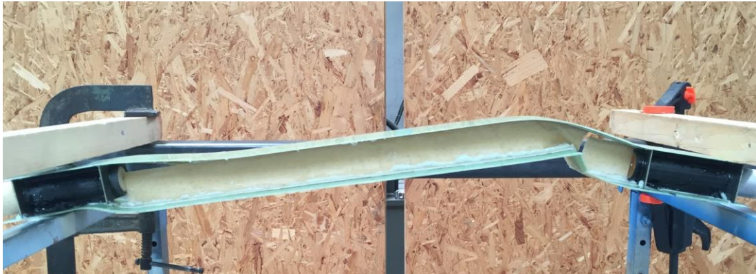
Figure 3.5: Failure of the spar.
