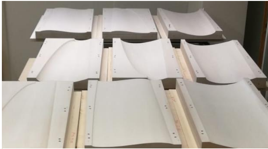
Figure 3.10: A view of some moulds of Titti's model undergoing surface treatment.
