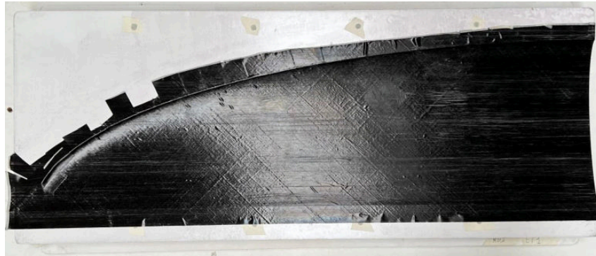
Figure 17: Carbon fiber fabric placed in the mold during lamination
